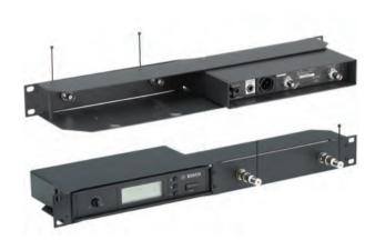
The kit is for mounting MW1-RX-Fx Wireless Microphone Receivers in 19" racks. It can mount two units, side by side in a one-unit high rack space. When only one unit is used, the other half of the frame can be fitted with the supplied panel, which can mount the two antennas. These are connected to the receiver via the two supplied BNC cables.
