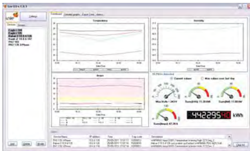
Monitoring Dashboards – shows all temperature, humidity and power sensors as trend lines for devices
