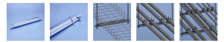
The Telescoping Strut Replacement is an innovative alternative to using strut-based trapeze or support structures to support cable tray, conduit or pipe. It eliminates the need for handling long lengths of strut and cutting sections of strut to size. The bracket telescopes to the desired length, attaches to threaded rod with a captive threaded nut at each end, and is locked in place by tightening a screw on a pre-installed steel band.
