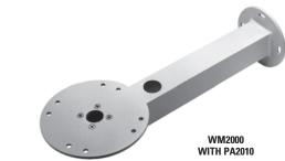
The **WM2000** is a universal wall mount designed for use with mediumand heavy-duty pan/tilts or enclosures. Constructed from aluminum, the **WM2000** will safely support up to 75 lb (34 kg). When used with the ST1 support strut, the maximum load is increased to 150 lb (68 kg). Optional mount adapters are available for corner, pole, and parapet applications.
