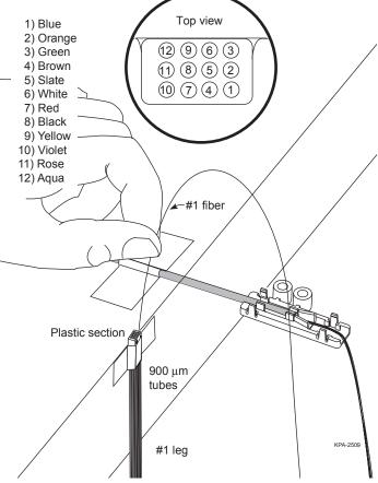
**Step 3:** Carefully thread about three inches of the first fiber into the #1 (blue) 900 micron tube.
