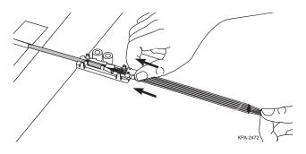
**NOTE:** At times the fibers will twist as a group when sliding the 900 micron assembly towards the
