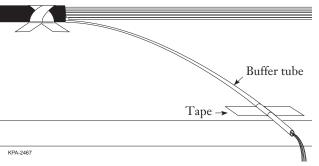
Step 4: If the buffer tube is gel-free, carefully cut out any water block yarns with scissors and skip to Step 6.
