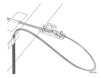
Step 7: Untape the 900 micron assembly from the table edge. Carefully slide the assembly while gently pulling the bare fibers protruding from the 900 micron tube ends until the assembly is above the fan-out body.
