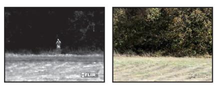
Thermal cameras can complement CCD cameras during the day in situations where contrast is low.
