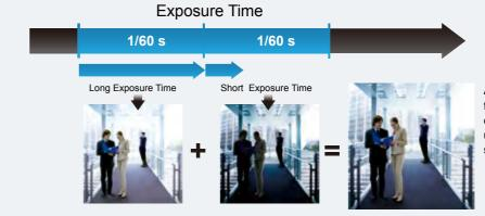
A single high-contrast frame is created by combining the two frames using an advanced image signal processor.
