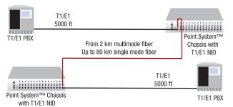
Devices must be used in pairs. Typical installation will include a chassis card installed in the Point System<sup>TM</sup> locally and a stand-alone device installed at the remote location.
