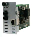
Connect central-office voice grade signals to distant Plain Old Telephone equipment (POTS) utilizing standard telephone signaling. Two units are required to implement an end to end system. Unit A connects to a telephone line or PBX and has the ability to detect ringing voltages and to act as a telephone (LINE SIDE FXS). Unit B is the reciprocal unit and has the ability to act as a Central Office and connects to a telephone device (CUSTOMER SIDE FXO).
