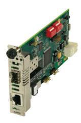
The T1/E1 copper to fiber network interface device (NID) provides a solution for those users that need to extend T1/E1 or PRI connections over fiber.
