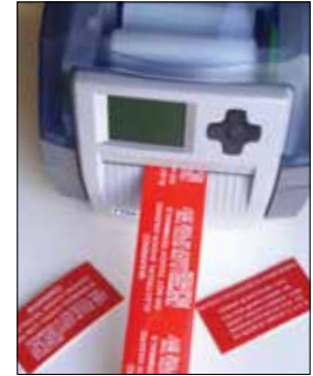
Using the suggested white ribbon, white text can be printed on red or black vinyl or a black ribbon can be used to print on the white vinyl.
