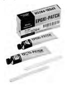
Applications include sealing rivets, bolts, metal joints, seams and welds, cement cracks, pipe couplings, joints, and tees. Each kit has two tubes of material, application instructions, and a mixing stick. When the resin and hardener are mixed, a gray epoxy is formed which cures at room temperature, has high adhesion, and will not sag. It is resistant to oils, acids, and chemicals.
