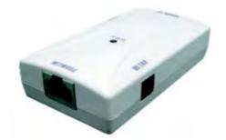
long power line that may cause any unexpected dangers to people. NPE-5818af is compliant with 802.3af PoE solution, it offers 48V/0.375A power supply with standard pin definition of Ethernet cable. Pin#1,2,3 and 6 with data transmission; pin # 4,5,7 and 8 with power enabled to device.
