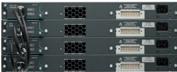
Figure 3. Cisco FlexStack Module and Switches
