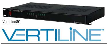
Altronix Vertiline8C CCTV Rack Mount Power Supply provides 8 fuse protected power outputs in a space saving 1U EIA 19" rack mount chassis which may be rack, wall or shelf mounted. This unit features individually selectable 24VAC and/or 28VAC power outputs with surge suppression. Vertiline CCTV Rack Mount Power Supplies are also available in sixteen (16) and twenty-four (24) output models with various power ratings.
