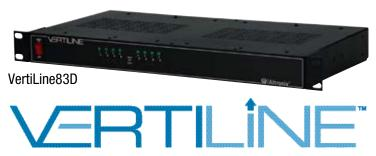
Altronix Vertiline83D CCTV Rack Mount Power Supply provides 8 PTC protected power outputs in a space saving 1U EIA 19" rack mount chassis which may be rack, wall or shelf mounted. This unit features individually selectable 24VAC and/or 28VAC power outputs with surge suppression. Vertiline CCTV Rack Mount Power Supplies are also available in sixteen (16) and twenty-four (24) output models with various power ratings.
