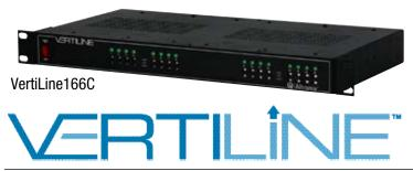
Altronix Vertiline166C CCTV Rack Mount Power Supply provides 16 fuse protected power outputs in a space saving 1U EIA 19" rack mount chassis which may be rack, wall or shelf mounted. This unit features individually selectable 24VAC and/or 28VAC power outputs with surge suppression. Vertiline CCTV Rack Mount Power Supplies are also available in eight (8) and twenty-four (24) output models with various power ratings.
