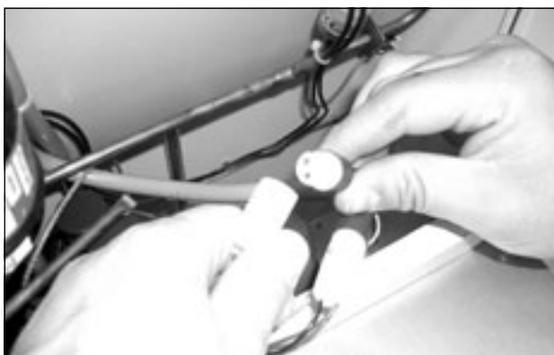
Fig. 74: Disconnect the fan connectors (3)
