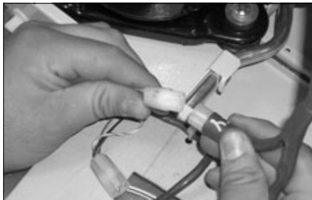
Fig. 50: Disconnect the fan connectors
