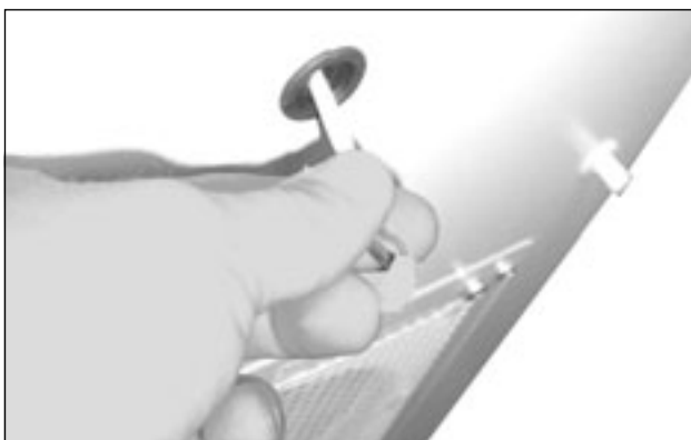
Fig. 68: Push back the display cable and press it through the cable gland (1)
