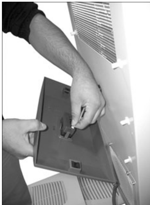
Fig. 45: Disconnect the connector from the display (1)
