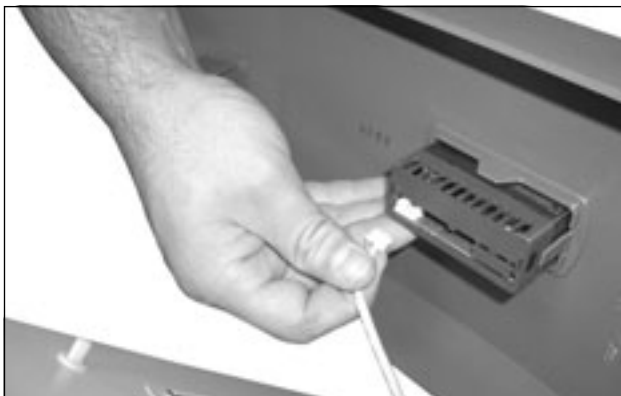
Fig. 67: Disconnect the display cable
