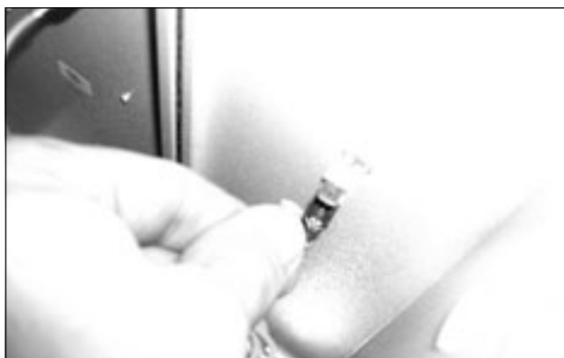
Fig. 76: Disconnect the fan earthing cable (2)
