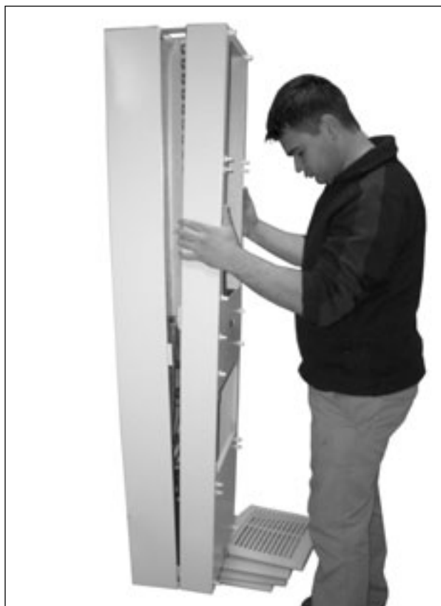
Fig. 78: Remove the cover
