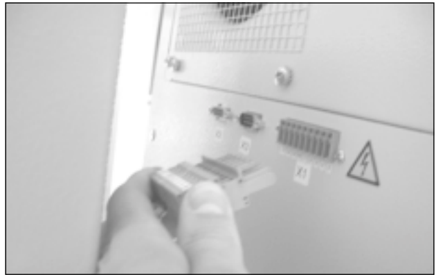
Fig. 41: Disconnect the power cord
