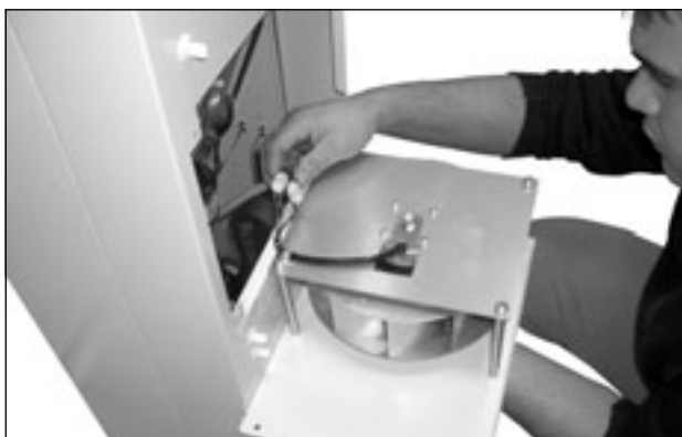
Fig. 72: Disconnect the fan connectors (1)
