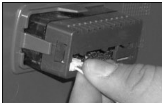
Fig. 46: Disconnect the connector from the display (2)
