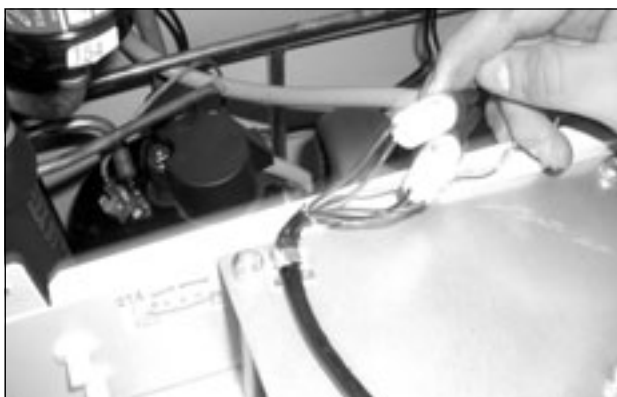
Fig. 73: Disconnect the fan connectors (2)
