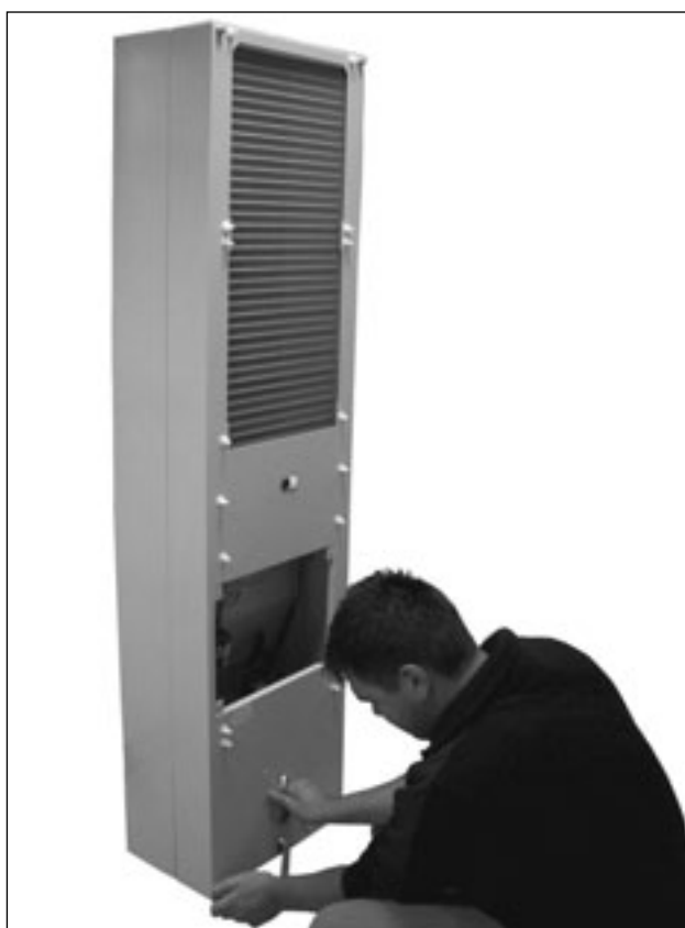
Fig. 77: Loosen the four screws of the cover
