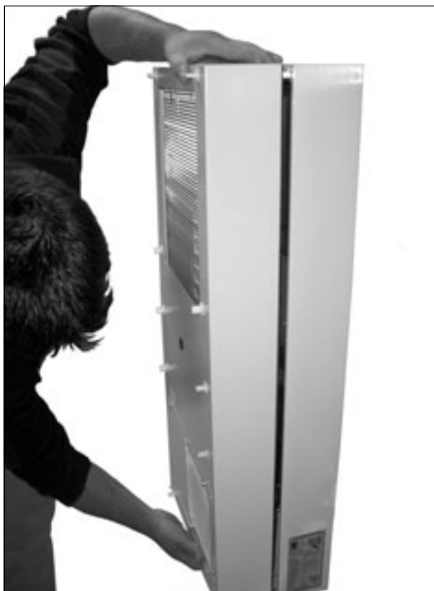
Fig. 54: Remove the cover (1)
