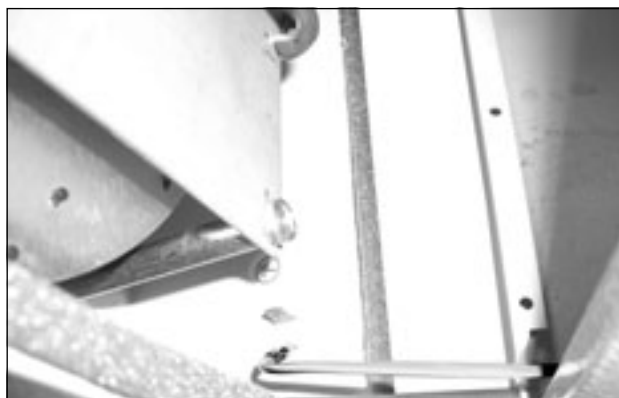
Fig. 56: Loosen the earthing cable between the cover and the chassis (1)
