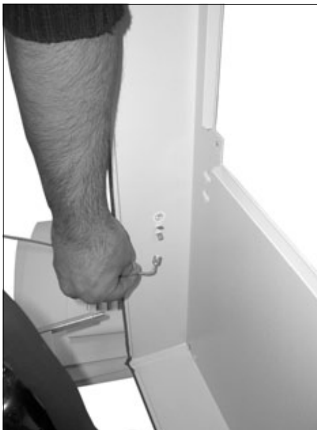
Fig. 80: Disconnect the earthing cable (2)
