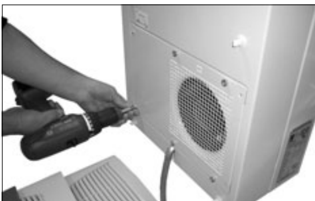
Fig. 48: Remove the external circuit fan (loosen the four screws)
