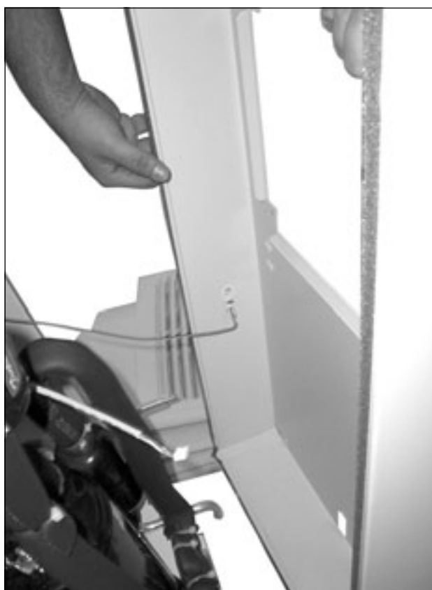
Fig. 79: Disconnect the earthing cable (1)
