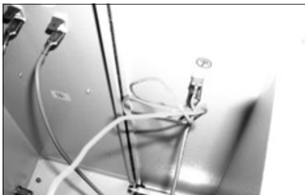
Fig. 75: Disconnect the fan earthing cable (1)
