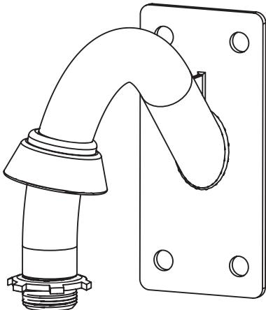
**Slide the grommet up the pipe and screw the conduit locknut to the top of the threads.**
