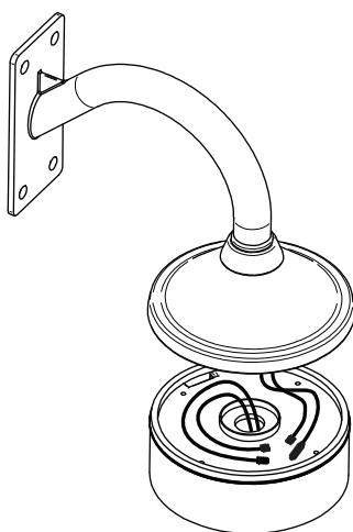
**Make electrical connections then coil excess wiring under the pendant cover.**
