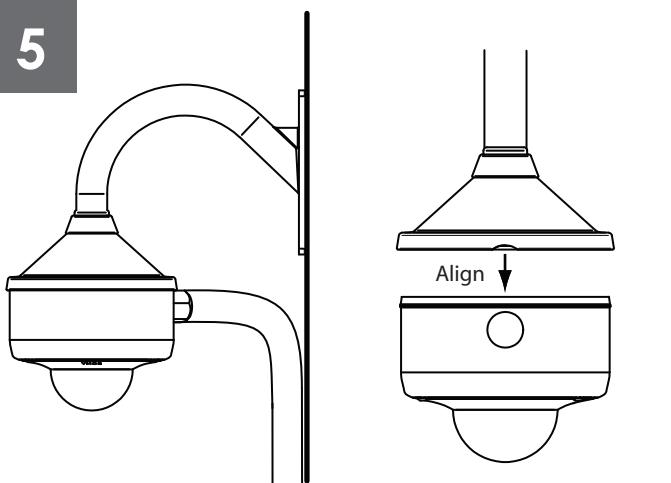
If applicable, the wiring may be run through a conduit. Take steps necessary to avoid water ingress when using a conduit.
