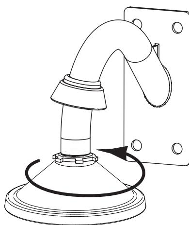
**Screw the pendant adapter snugly onto pipe. Tighten locking nut.**
