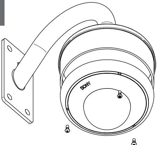
**Attach the dome assembly to the housing with security screws. Complete all wiring connections.**
