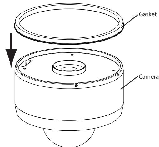
**Fit the provided gasket into the circular groove on the camera base as shown.**
