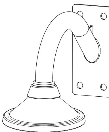
**Pull the rubber grommet down over the locking nut as shown.**
