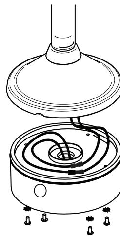
**Attach the mid-section of the housing to the top with the (4) screws and star washers.**
