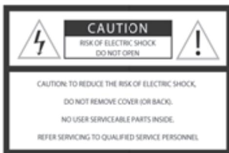
The lightning flash with an arrowhead symbol, within an equilateral triangle, is intended to alert the user to the presence of non-insulated "dangerous voltage" within the product's enclosure that may be of sufficient magnitude to constitute a risk of electric shock to persons.
