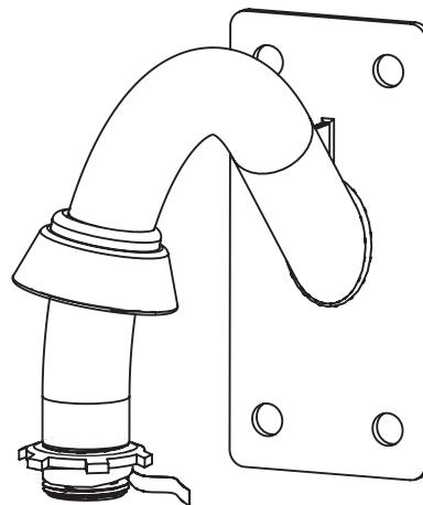
**Wrap Teflon tape around pipe threads to ensure a water tight connection.**
