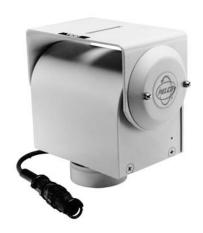
The **PT270-24P** "mini" pan/tilt has been carefully engineered to accommodate the lighter, smaller, new generation of CCTV cameras. Small in size, but rugged in operation, the **PT270-24P** measures only 7.75 inches (19.69 cm) high, 8 inches (20.32 cm) wide, and 4.50 inches (11.43 cm) deep. Ideally suited for indoor operation, this pan/tilt can be used in discreet enclosure applications or where space is a consideration.
