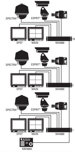
\*INCLUDES BUILT-IN RECEIVER FOR CONTROL OF PAN/TILT/LENS FUNCTIONS. OTHER PAN/TILT UNITS MAY REQUIRE SEPARATE RECEIVER.
