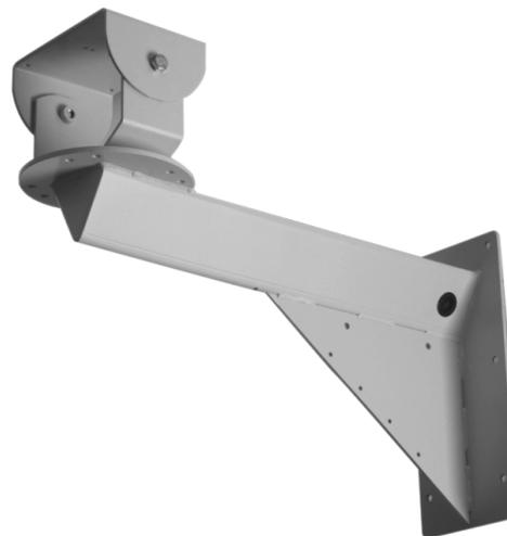
The **WM3026** wall mount has been designed specifically for use with Pelco's heavy duty pan/tilts and/or enclosures. Manufactured from 0.25-inch (6.35 mm) aluminum, the **WM3026** is capable of supporting a maximum load of 300 pounds (136.08 kg) and can be safely mounted to any vertical load-bearing surface.
