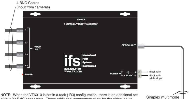
of four (4) BNC connectors. These additional connecttors allow for the video inputs to be inserted from the front OR back of the unit BUT NOT BOTH.
