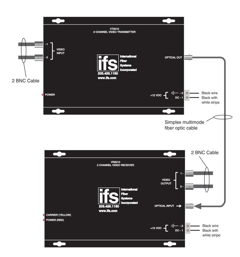
NOTE: WITHOUT PROPER FIBER CONNECTION, LED'S DO NOT INDICATE CORRECT OPERATIONAL STATUS OF THE UNIT.
