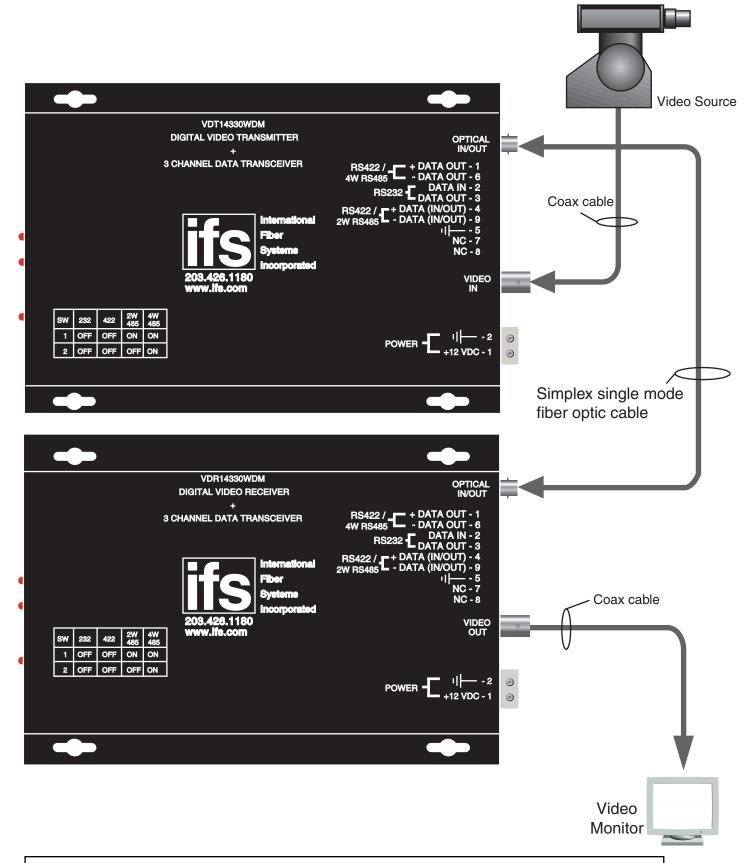
NOTE: WITHOUT PROPER FIBER CONNECTION, LED'S DO NOT INDICATE CORRECT OPERATIONAL STATUS OF THE UNIT.
