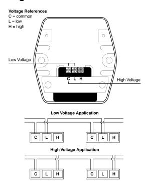
**Important:** When you connect the wiring for the single-coil or double-coil 24/120 door holder, attach the green wire to the earth ground.
