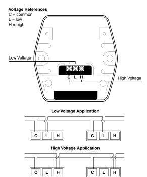
**Important:** When you connect the wiring for the single-coil or double-coil 24/120 door holder, attach the green wire to the earth ground.
