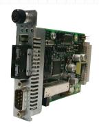
Ideal for campus or business environments where remote devices can be networked in a point to-point configuration and distances are greater than the 15 m limitation of conventional copper serial cables.
