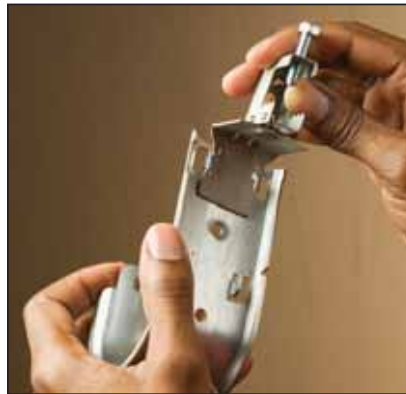
Step 2: Hook the Angle Bracket assembly into the J-Hook and press-fit into position
