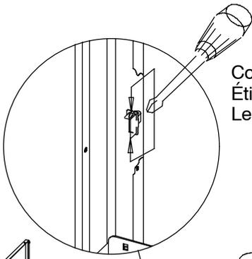
Compress tabs for latch removal
