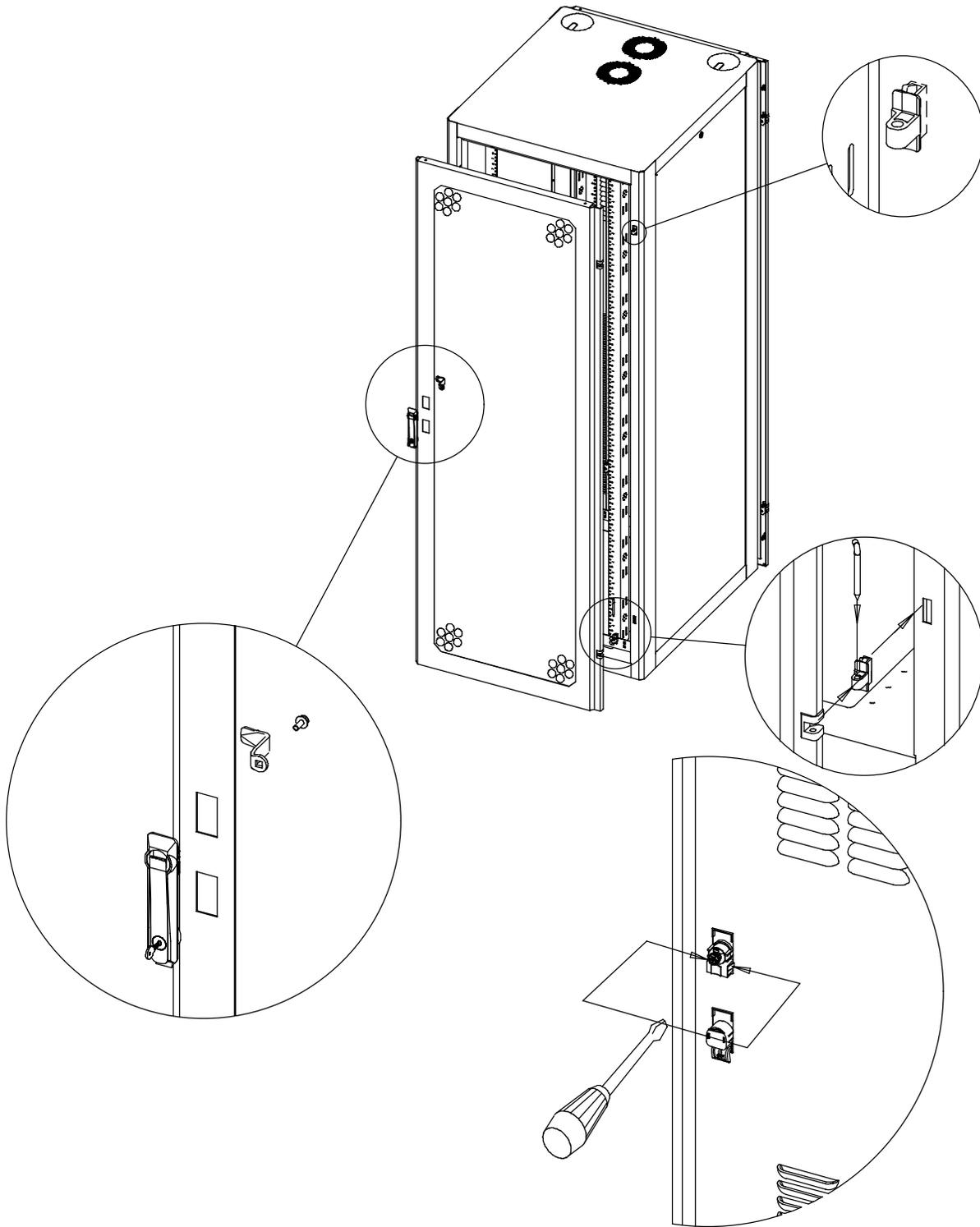
Compress tabs for latch removal
