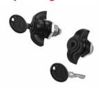
Keylocking quarter-turn wing knob latch. Black finish. Includes gasket, mounting nut and one key with 333 key code. Use existing cam for installation; cam is not included with wing knob. Can be locked in open or closed position. Maintains cabinet rating Type 4, 12.
