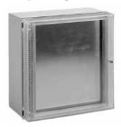
Clear molded polycarbonate window has a 31.8-mm (1.25-in.) clear space between enclosure front opening and window surface. Space also accommodates equipment mounted on optional front plate. Window kit is hinged on left side with a 140-degree door opening and a quarter-turn slotted latch. Includes mounting hardware for
