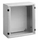
Aesthetic die-cast frame has .125-in.-thick clear polycarbonate window. Preassembled kit is secured to front opening of enclosure by mounting screws. Window frame caps conceal mounting screws. Frame has RAL 7035 light-gray textured polyester powder paint finish.
