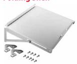
The shelf mounts to door using the Door Bar Grid Straps (sold separately). Shelf is 16 gauge steel with 12 gauge brackets. Shelf finish is RAL 7035 textured light-gray polyester powder paint. Locks in two positions—90 degrees as a shelf and 15 degrees as a writing surface. Also mounts to three-row grid straps, side or back panel, or any flat surface. Holds up to 30 pounds.
