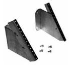
Swiveling rack angles drop 45 degrees to provide convenient access to equipment mounted on patch panel location in 36- and 48-in. (914and 1219-mm) high cabinets. Made of self-grounding, plated 12 gauge steel. Mounting hardware included. Set of two.
