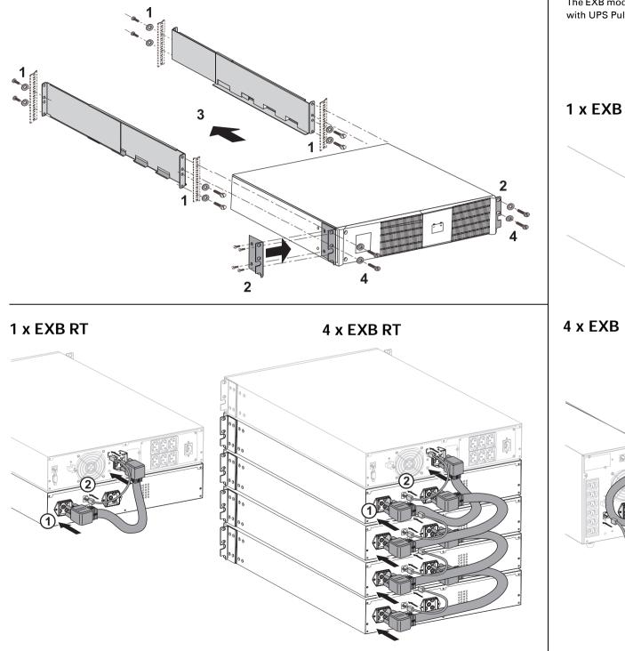
The EXB models EX EXB 1000/1500 and EX EXB RT2U 1000/1500 must be used together with UPS Pulsar series models EX 1000, EX 1000 RT2U, EX 1500 and EX 1500 RT2U.
