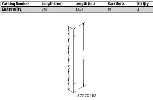
Provides 19 RU. Allows use of most 19-in. rack-mount accessories. See Selected Networking PC Cabinet Accessories. Package includes two rack angles and mounting hardware. Required for accessories noted in Selected Networking PC Cabinet Accessories table; not compatible with EPCEQS Shelf.
