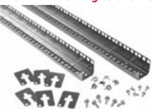
PROLINE® Rack Angles are available in 19-, 23- and 24-in. configurations. All Rack Angles have two mounting surfaces that serve as mounts for both rack equipment and rack accessories. Rack Angles are furnished in pairs and are available with tapped holes that directly accommodate 10-32 screws or square holes for use with cage nuts and M5, M6 or 10-32 screws. Rack Angles comply with ANSI/EIA RS-310-D rack mounting standards.
