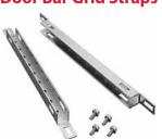
Straps mount to the door bar. Used to mount accessories to the door. Constructed of 16 gauge steel with plated finish. Holds up to 100 lb. Bulletin: P20
