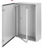
Swing-Out Rack Frames provide 120-degree swing-out access for 19-in. rack equipment. Welded rack frame mounts to front flange. Distance from frame to door surface is 1.32 in. (33 mm) for solid doors and 1.07 in. (27 mm) for window doors. Frame is painted white. Mounting hinge and latching hardware provided. Order separately clip nut package catalog number XNM5 and screws
