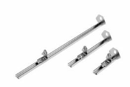
Adjustable-Depth Mounting Kits provide mounting means for installing panels, swing-out panels, DIN rails, rack angles, mounting channels or grid straps at any depth from front to rear of enclosure. Kits include slide mechanisms and hardware. Use two kits when enclosure has 6 collar studs for mounting panel. Dead Front Panel and Swing-Out Rack Frame cannot be mounted on
