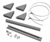
Adjustable-Depth Mounting Kits provide mounting means for installing panels, swing-out panels, DIN rails, rack angles, mounting channels or grid straps at any depth from front to rear of enclosure. Kits include slide mechanisms and hardware. Use two kits when enclosure has 6 collar studs for mounting panel. Dead Front Panel and Swing-Out Rack Frame cannot be mounted on adjustable mounting kit.
