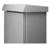
Solar Shield Top provides a vented area on top of the enclosure to absorb solar heating effects and help keep enclosure cool. Also provides a drip shield to keep liquids away from the door sealing surface. Aluminum with RAL 7035 textured light-gray finish inside and out. Maintains enclosure rating. Includes mounting hardware.
