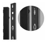
PROLINE® combination vertical cable manager provides increased versatility for power and cable management for 2000-mm tall frames. Tool-less mounting with key hole slots accept many vertical PDUs (APC, Geist, etc.). Flush arrowhead cutouts provide convenient cable manager tie-down points. Hardware and ten VELCRO® cable wraps included. Finished with RAL 9005 black polyester powder finish. VELCRO is a trademark of Velcro Industries B.V.
