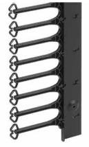
Fingers separate, support and manage cable. Bracket mounts on either left or right side of 700- and 800-mm cabinets between the frame and the rack angle to create vertical wiring space. Bracket has RAL 9005 black polyester powder paint finish. Fingers are molded black plastic. Mounting hardware included.
