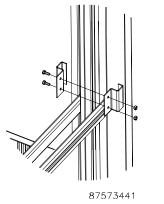
Allows two network cabinets to be joined together. Requires removal of side covers on both joined cabinets. Brackets are used in pairs. Includes eight brackets and mounting brackets.
