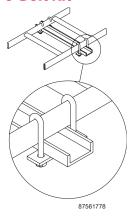
Connects ladder rack to top of cabinet or to auxiliary support channel. Each kit includes two J-bolts and makes one support connection. Kit components are plated steel. Includes mounting hardware.
