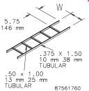
Supports cable on straight runs. Made of 1-1/2 in. x 3/8 in. (38 mm x 8 mm) 16 gauge tubular steel with a painted or plated finish. Nominal installed length is 10 ft. (3.05 m). Each section is 9 ft. 11-1/2 in. (3.03 m) long with cross members welded at 9-in. (229-mm) intervals.
