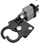
Provide a means of using two padlocks on a secured power source. Either padlock can be removed enabling power to be interrupted and enclosure accessed. Catalog number ASLDAC includes a 10.00-in. (254-mm) plated steel chain. Lockouts are manufactured from 10 gauge steel and finished in red. Padlock holes are .38-in. (10-mm) in diameter. Padlock is not included.
