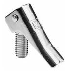
Provides quick access to Type 4 and 4X floor-mount and free-stand enclosures with clamps. The 3/8-16 threaded, stainless steel toggle latches replace the standard stainless steel bolts. Operation of the toggle releases the door clamp so the door can be opened without tools. Two Type 316 stainless steel toggle assemblies included.
