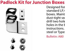
Designed for field installation on standard LP, CH and CHNF junction boxes. Maintains water-tight and dust-tight seal. To install simply drill two holes in the cover and two holes in the body. Includes complete instructions. Padlock Kit is plated steel or Type 316 stainless steel.
