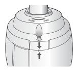
5. Attach Camera Turn the camera frame counterclockwise until
