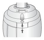
5. Attach Camera Turn the camera frame counterclockwise until the protrusions on the camera frame and installation base become matched perfectly.
