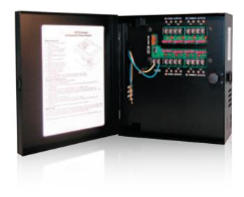
The PWR-24AC-4-4UL is a UL listed CCTV power center engineered to manage remote camera and accessory power requirements. The PWR-24AC-4-4UL distribution module is designed with 4 individually fused outputs for powering up to 4 CCTV cameras and accessories. It will provide 24Volts AC via distribution to four fused outputs with a total of 4.0 Amps continuous supply current. The PWR-24AC-4-4UL power center is housed in a premium heavy gauge metal enclosure.
