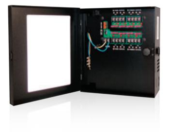
The PWR-12DC-8-5 is a CCTV power center engineered to manage remote camera and accessory power requirements. The PWR-12DC-8-5 distribution module is designed with 8 individually fused outputs for powering up to 8 CCTV cameras and accessories. It will provide 12 VDC via distribution to eight fused outputs with a total of 5 Amps continuous supply current. The PWR-12DC-8-5 power center is housed in a premium lockable heavy gauge metal enclosure.
