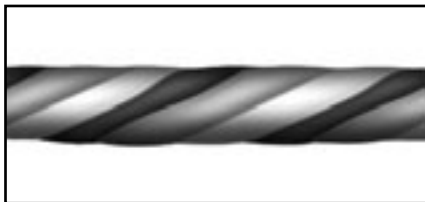
Twisted wires minimize disruptive AC magnetic fields
